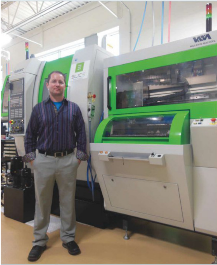
Michael Rappach, VP manufacturing, stands in front of Slice Mfg. Studios' Willemin 508 MT machining center used for finish machining the hip cups.
